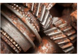
relative humidity at 49°C (120°F), the protective oil film provides 3-7 days outdoor protection on polished steel or sand-blasted panels. For extended or outdoor storage protection, use NuKoat HPO. Provides 3-9 months indoor protection on steel and cast-iron.
