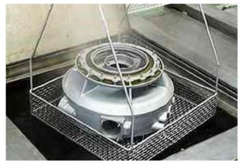
**AquaKlean EF105MF** was formulated to provide improved removal of particulates and organics while providing reduced residues, and fast rinsing. **AquaKlean EF105MF** provides excellent wetting and rinsing properties and is therefore an excellent choice for pre-plate cleaning. Removes: inks, polishing and buffing compounds, grease, oils, fingerprints, drawing compounds, and metalworking fluids.
